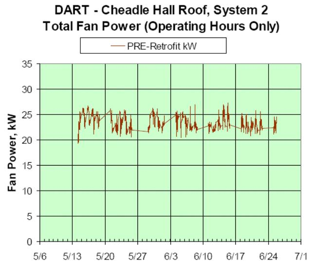
**Figure 1 Fan Power Loading Pre-DART**
